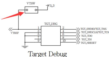
In case that the target board requires 20-pin 0.05" JTAG header or some none standard connector, you can always easily bridge the IBDAP TGT\_DBG connector over using the IBDAPC10J20 ARM 20-pin 0.1" to Cortex 10-pin 0.05" JTAG/SWD Adapter which is included in the IBDAP product.
